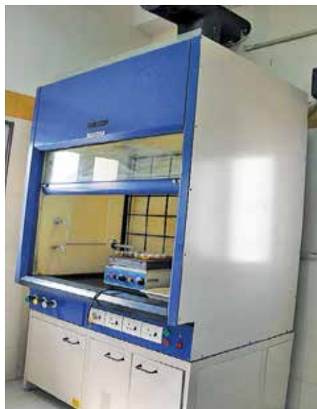
Fig. 10.4 Fume hood chamber
