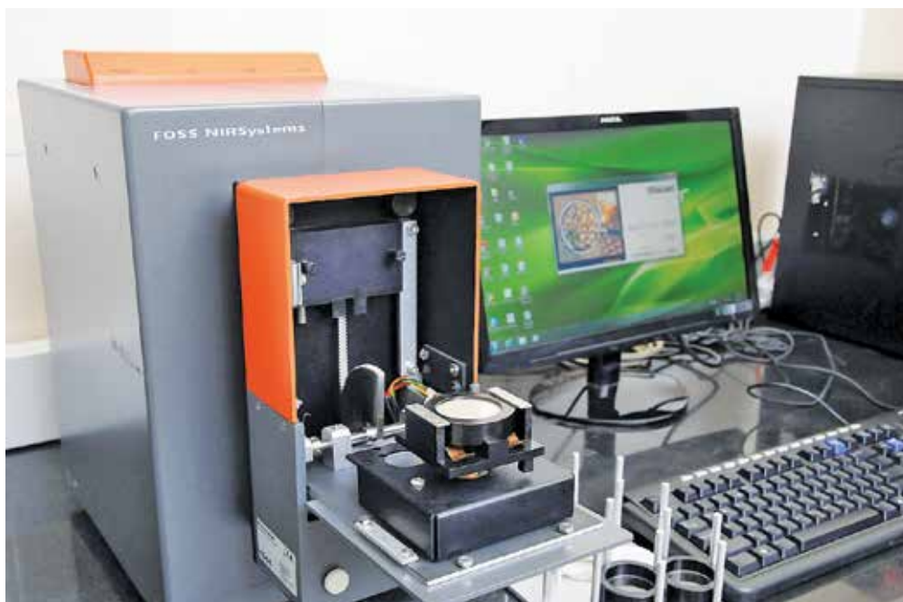
Fig. 7.14 Near infrared analyzer
