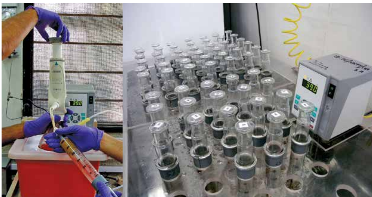
Fig. 13.1 Incubation of samples by in vitro gas production technique
