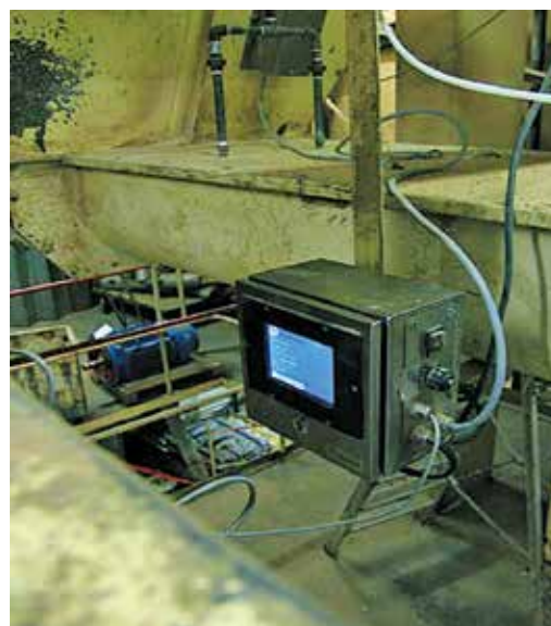
Fig. 3.21 Moisture meter installed in a conveyor
