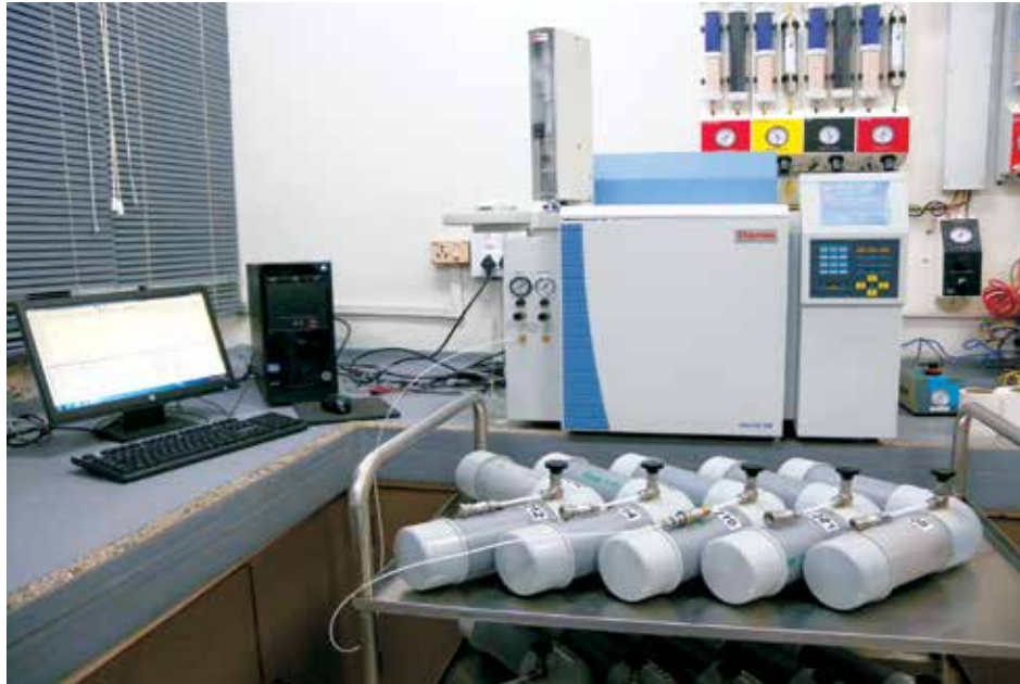
Fig. 18.5 Breath sample analysis using GC
