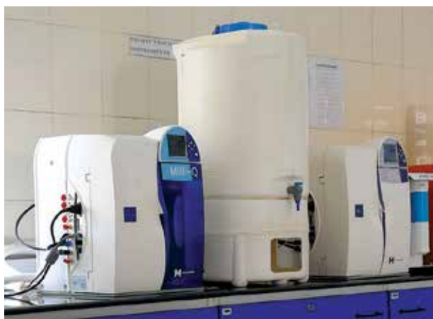
Fig. 6.4 Water purification system
