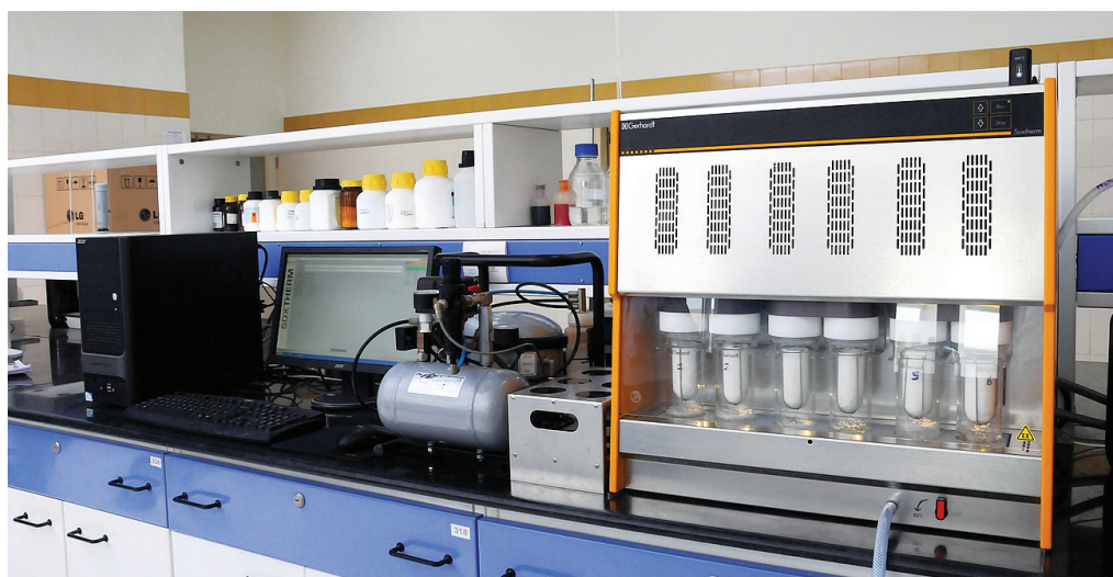
Fig. 7.9 Fat extraction by Soxtherm
