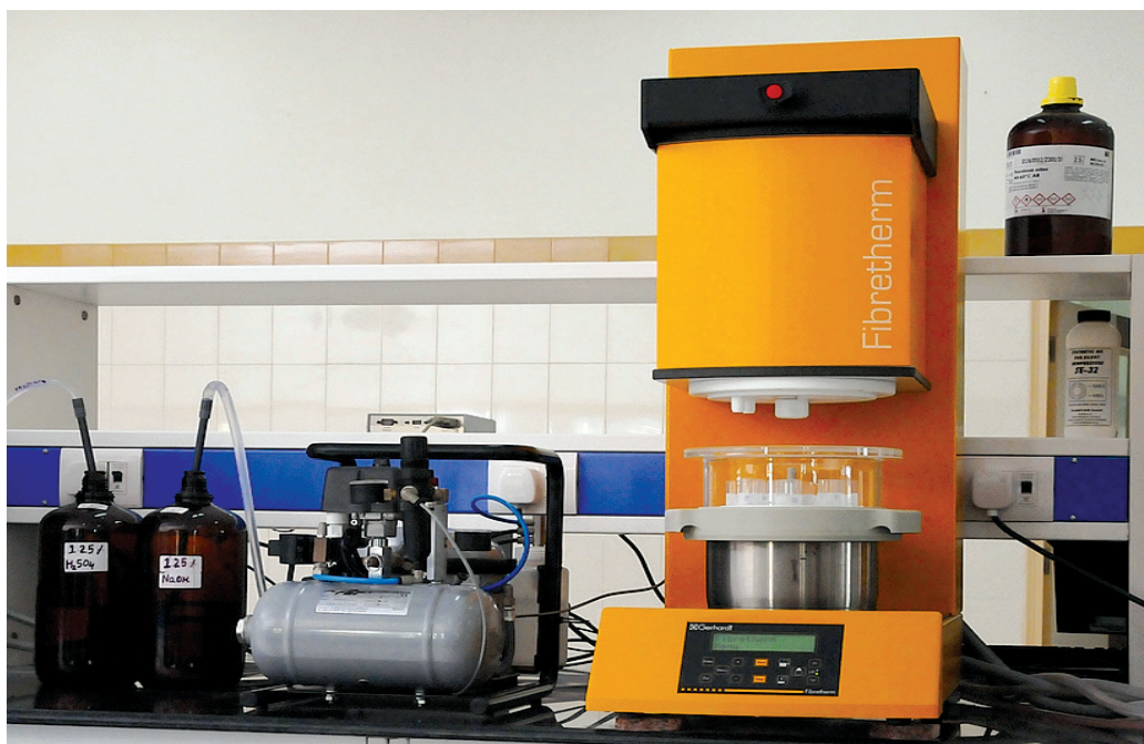
Fig. 7.10 Crude fibre estimation by Fibretherm
