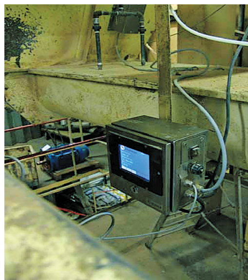
Fig. 3.21 Moisture meter installed in a conveyor
