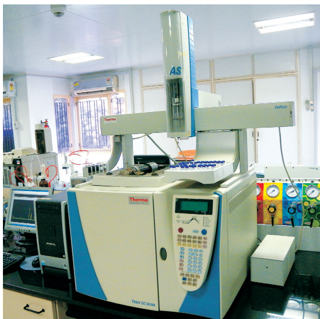
Fig. 17.1 Pesticide residues estimation by GC
