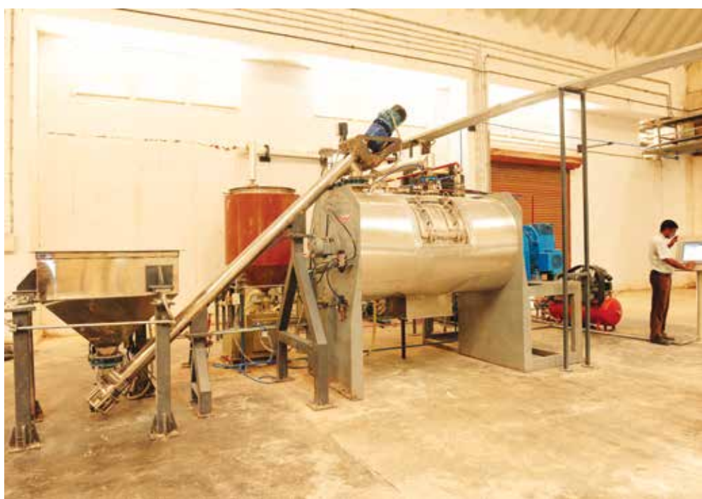
A bypass fat plant for production of bypass fat supplement
