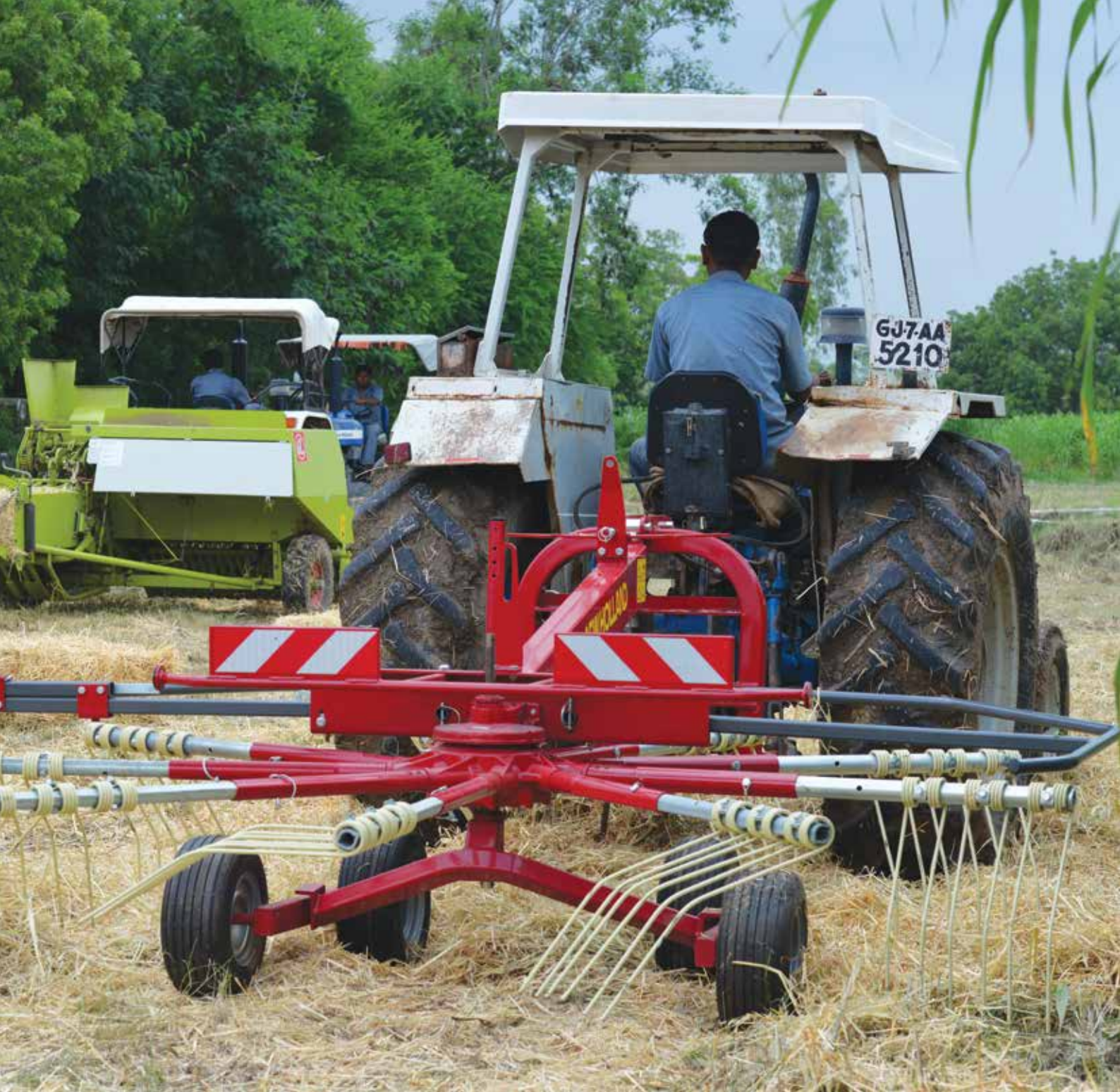
Straw collection rake for faster sun drying of succulent bio-mass
