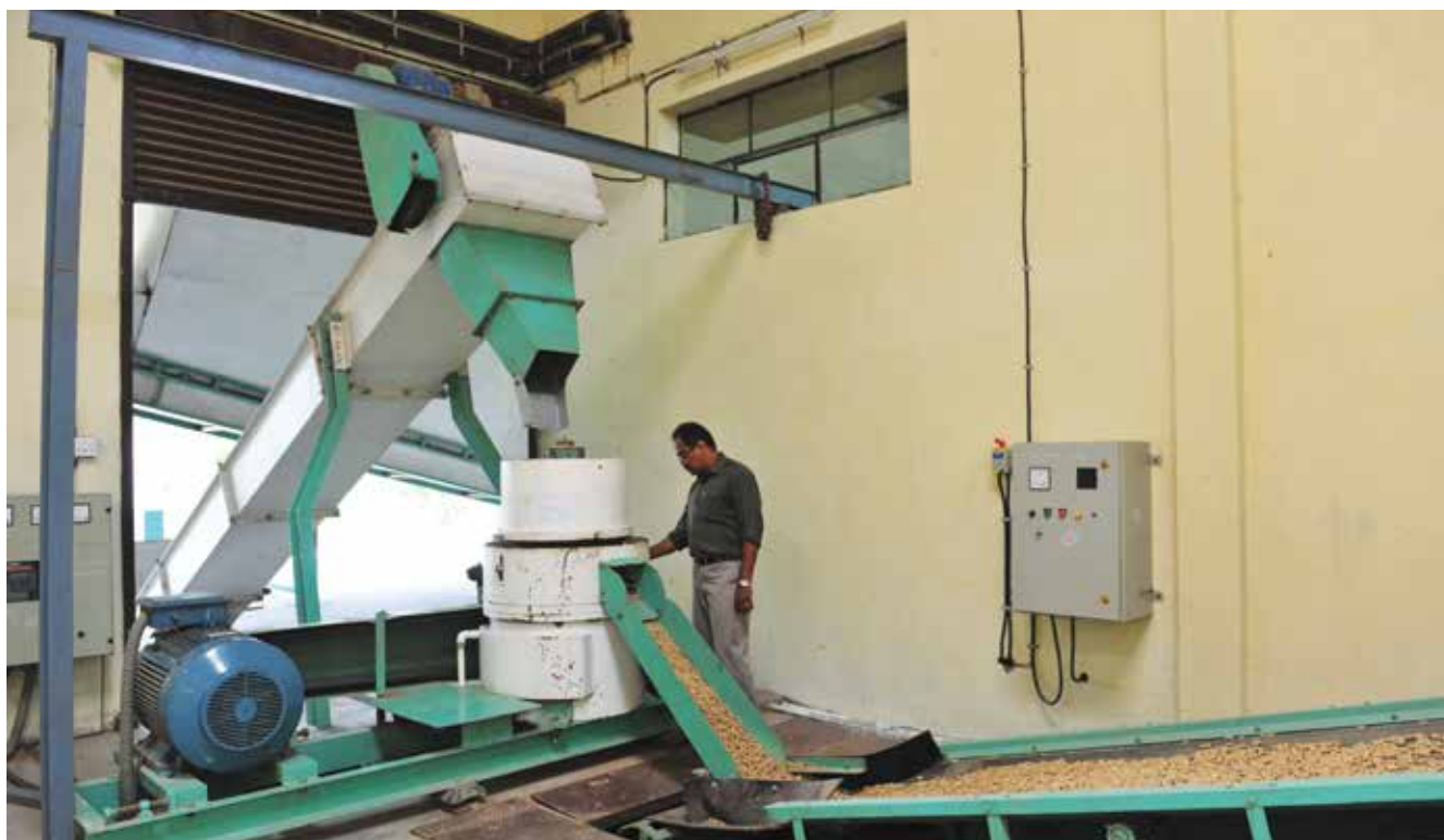
Manufacturing enriched straw based feed pellets
