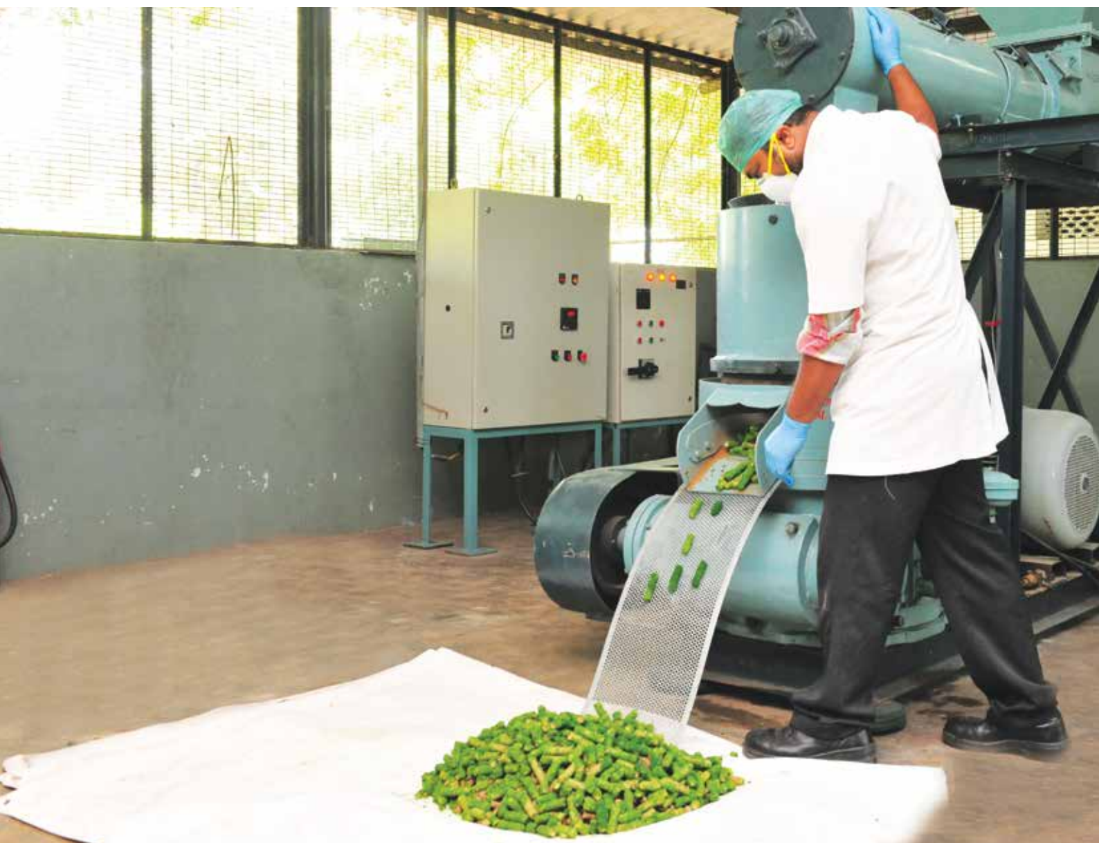
Pilot scale production of straw based feed pellets
