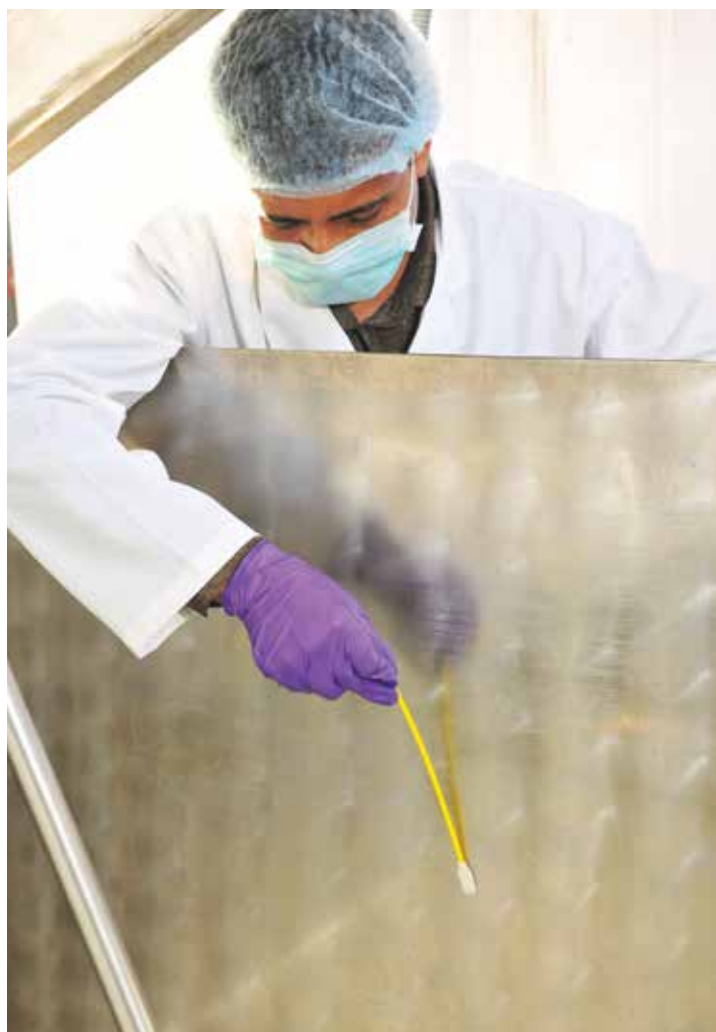
Checking the efficacy of newly developed chemical formulation in cold cleaning of bulk cooler
