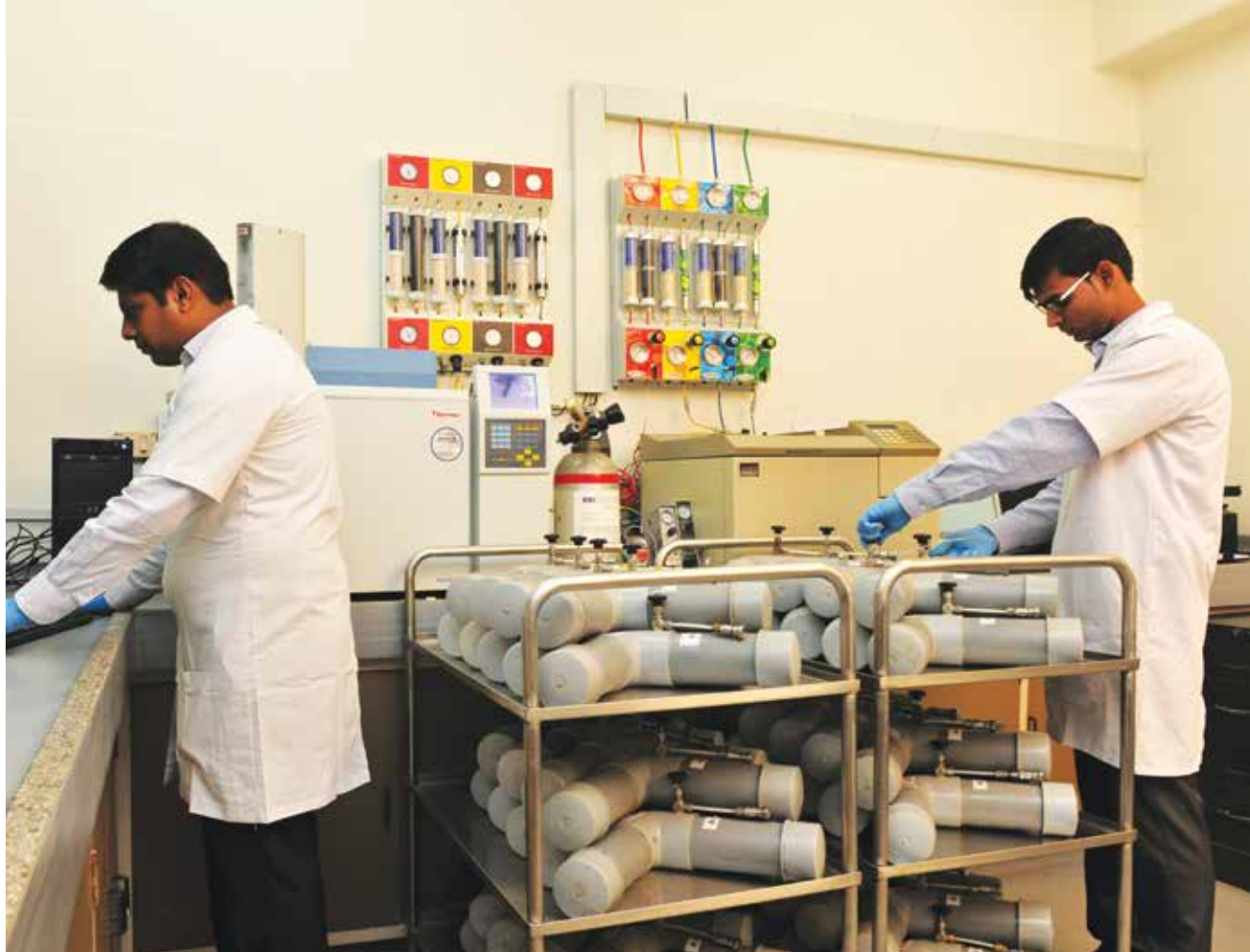
Methane measurement using Gas Chromatograph in breath samples collected in canisters from field animals
